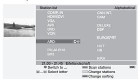
For an alphabetical display: Enter letters with the numeric button (like on a mobile phone keypad), select with  $\checkmark \land \checkmark$  and call with **OK**.
